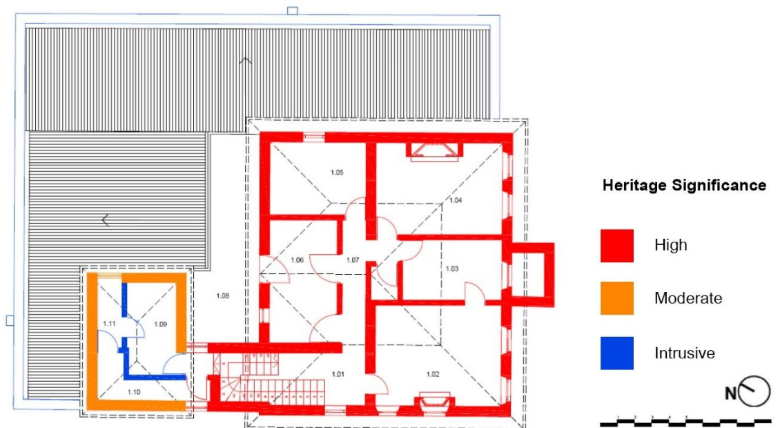
Figure 88 — Heritage significance of built fabric focussed on the eras of construction. Scale: 1:200
