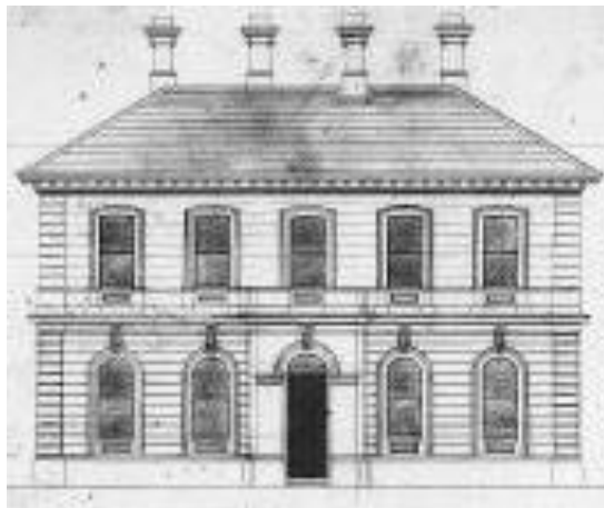
Figure 90 – Street elevation of the former Bank of New South Wales branch, Bathurst, by Edmund Blacket. This was among the first three branches design 1856–59 for the Bank of New South Wales by Blacket. The similarity with the CBC branch at Campbelltown shows how this early model influenced the design of many architects designing for many bank clients in the second half of the Nineteenth Century. (source: Mitchell Library, D215–1; 41)
